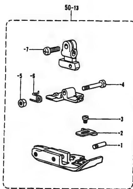
D. 押工脚体/Presser foot mechanism/Stoffdruckertuls/
