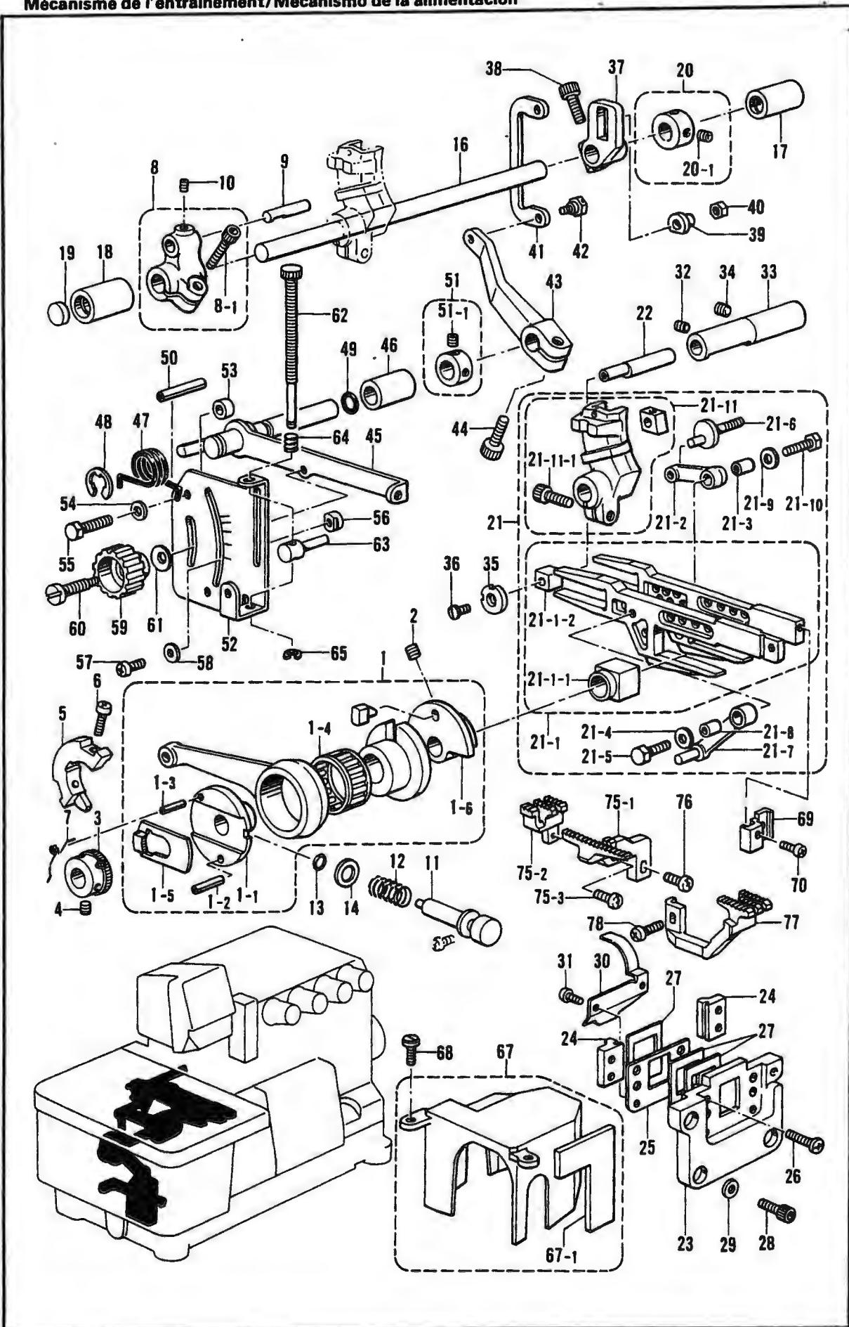
E. 送り関係/Feed mechanism/Transportvorrichtung/
